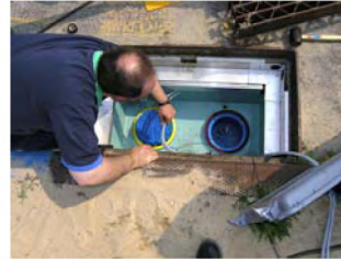
StormBasin bacteria testing at a beach parking lot
