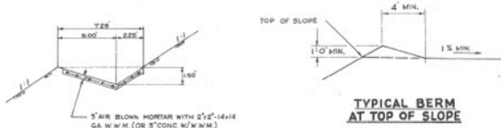
TYPICAL TERRACE DRAIN SCALE: 1/2" = 1'-0"
